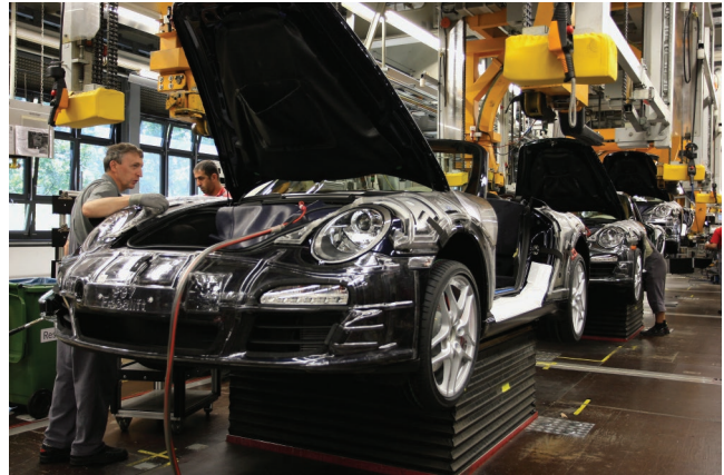
Automobile assembly lines use a product layout.
