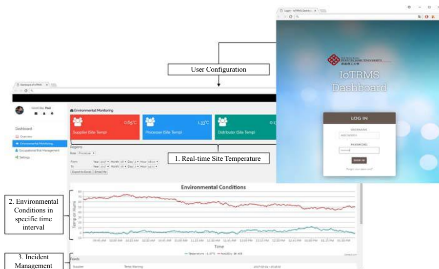
Figure 16. User interface of environmental monitoring in IoTRMS
