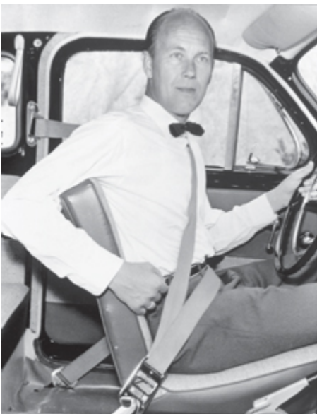
Volvo inventor Nils Bohlin created the original three-point seat belt—and then shared it with the world.
